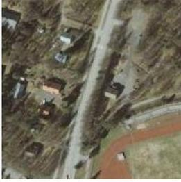
NLS orthophotos are an aerial photo data set covering the whole of Finland. The geometry of the orthophotos corresponds to a map. The terrain resolution is 0.5 m. Some 0.25 m orthophotographic data is also produced in conjunction with laser scanning flights. NLS orthophotos are updated every 3 to 10 years. The product is a part of the NLS raster material.
